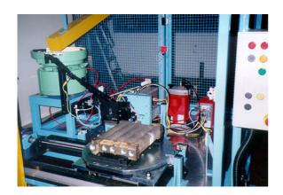
This rig is designed to handle two cast heat exchangers. The machine automatically applies adhesive and inserts core plugs, one at a time, into ten machined holes.
