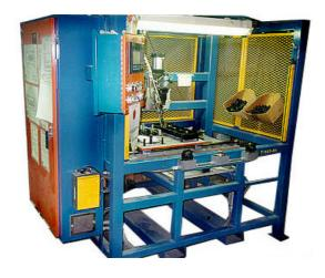
This machine is another example of the application of automatic adhesive dispensing. The adhesive is a 2 part mix supplied from 210 litre drums, which are to be kept at a controlled temperature. The dispensing gun mixes the constituents in the required proportions before being deposited as a gasket pattern to the parts.
