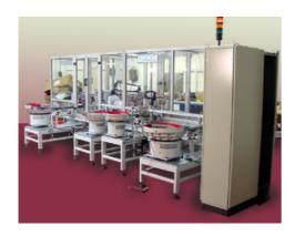
The facility is completely guarded with aluminium extruded frames and clear guard panels. All of the openings for the bowl feeders are outside the guarded area, allowing the operator to top up the bowls without stopping the machine. The deposit point for the assembled and tested product is also outside of the guarded area. The carton filling system also has an automatic carton change facility.
