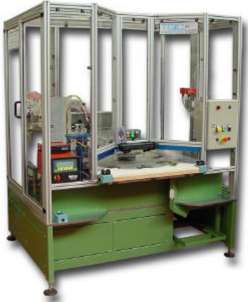
Manually Loaded/Unload Machine Operating on an 8 second cycle
